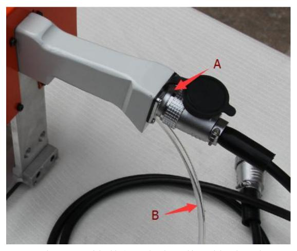
A: connect the 19 core aerial cable (one end to the machine and the other to the controller)
