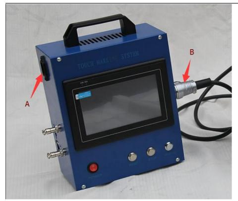
A: controller power line interface (need to ground wire, otherwise long term use will cause harm to display)
