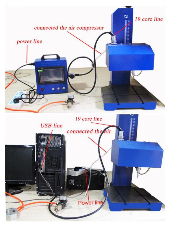
A: connect the 19 core aerial cable (one end to the machine and the other to the controller)
