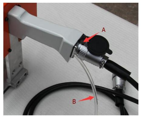
A: connect the 19 core aerial cable (one end to the machine and the other to the controller)
